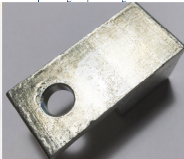
After spreading drop over lug contact surface
