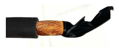
**4.** If the flex wire is NEAR TO the maximum capacity of the lug and especially true for type K "hairy" wire, <u>use a wire tie or a turn of electrical tape</u> at the end of the stripped cable to control the strands before and while inserting the wire in the wire hole. Snip off the wire tie or pull the tape out of the rear sight hole before tightening the binding screw.
