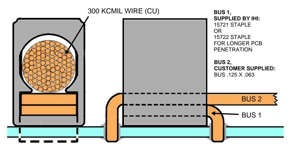
WHEN USED WITH A SINGLE PCB LEG THE UPPER BUSBAR NEEDS TO BE ANCHORED IN A WAY TO PREVENT THE LUG BODY FROM ROTATING WHEN THE WIRE BINDING SCREW IS TORQUED AND FROM SLIDING WHEN WIRE IS PULLED. FULL LINE CURRENT FROM WIRE IS SPLIT 50/50 BETWEEN TWO BUS LOADS, 1 AND 2.
