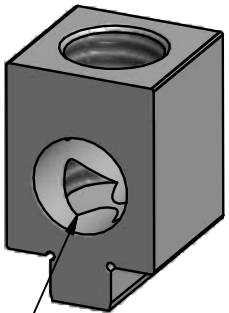
Figure 2: Less Sturdy: Horizontal screw and horizontal wire. Best for factory wiring only. Figure 3: Least Sturdy: Horizontal screw and vertical wire. Best for factory wiring only.
