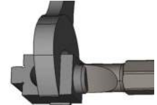
Figure 2: Less Sturdy: Horizontal screw and horizontal wire. Best for factory wiring only. Figure 3: Least Sturdy: Horizontal screw and vertical wire. Best for factory wiring only.
