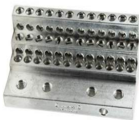
36S4-3 WIRE BODY. 36 WIRE HOLES, 4-14 AWG, TWO MOUNTING BOLT HOLES, CLICK TO SEE MORE ON PAGE 7
