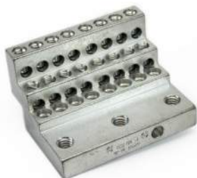
"24S4-3" WIRE BODY. 24 WIRE HOLES, 4-14 AWG, TWO MOUNTING BOLT HOLES. CLICK TO SEE MORE ON PAGE 6
