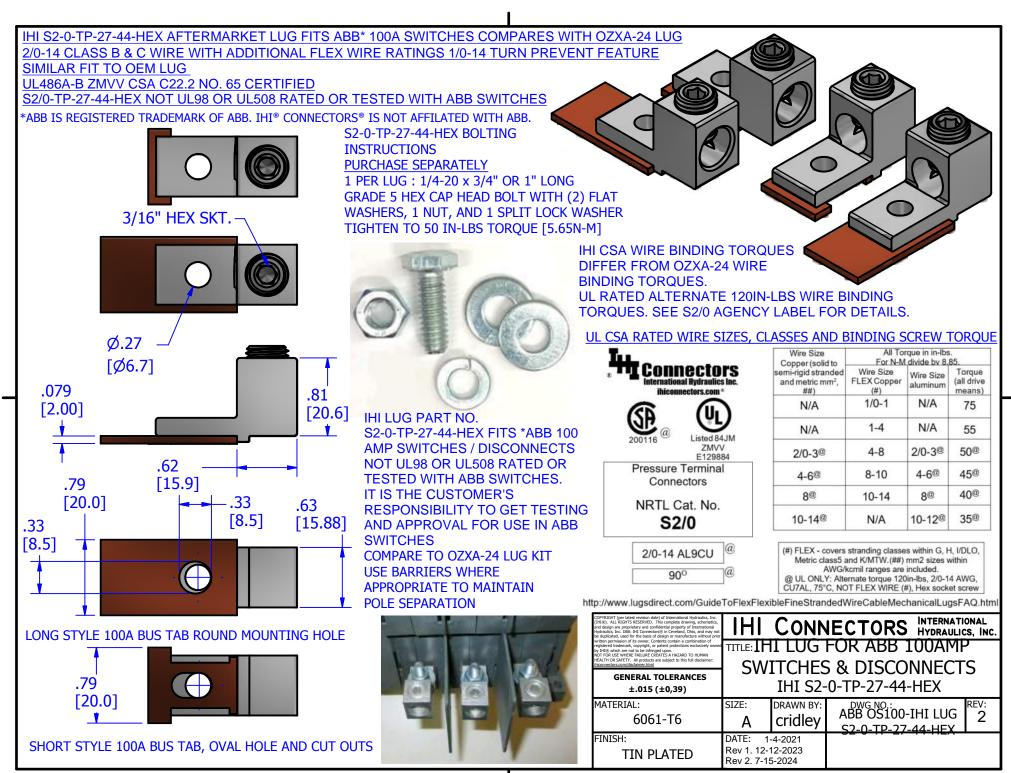
FOR DETAILED LUG DIMENSIONS AND SPECS SEE LINK https://lugsdirect.com/PDF\_Webprint/S2-0-TP-27-44-HEX%20%20(WEB).pdf
