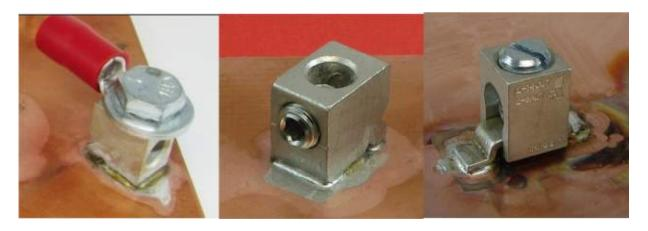
The typical edge fillet on the IHI Solderable terminal in SMT mode is about .025" rad. (varies with amount of solder/paste used) so we suggest that the copper pad showing through the masking would be .050" total wider than the physical contact footprint to accommodate the .025" all around.
