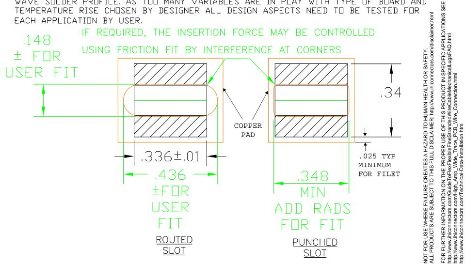
SOLDER FOOT PRINT FOR IHI B6A-PCB-XX, B6A-NH-PCB-XX, & B6A-PCB-45-XX
